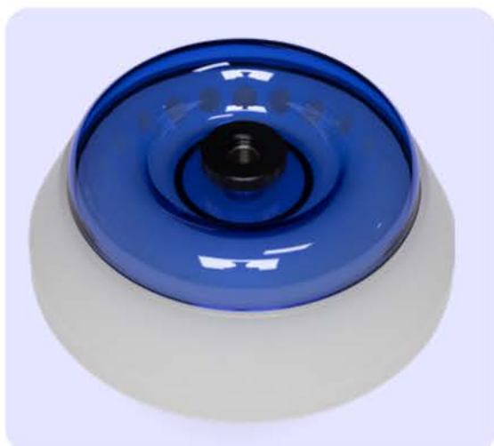
C-R-FA5424 rotor with included sealed lid.
