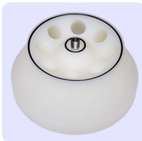
C-R-FA5308 rotor without included sealed lid.
